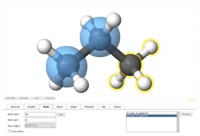
Figure 1. Structure mapping tool. Mapping a propane molecule to a three bead coarse-grained molecule. The beads are displayed in blue. Atoms surrounded by the yellow circles are selected and about to be mapped to a bead.
