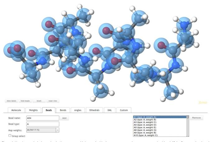
Figure 6. Mapping a polyalanine molecule. Heavy atoms with its attached hydrogens are mapped to one coarse-grained bead. [Color figure can be viewed in the online issue, which is available at wileyonlinelibrary.com.]
