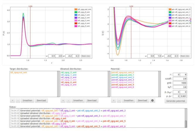
Figure 7. Coarse-graining water molecules. The figure shows part of the process of creating effective potentials for TIP3P water molecules. Reduced units are used in the figure. [Color figure can be viewed in the online issue, which is available at wileyonlinelibrary.com.]
