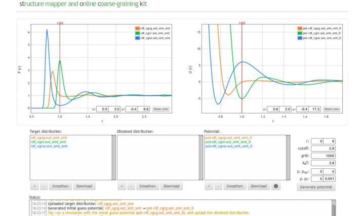
Figure 3. Boltzmann inversion tool. In the above figure, RDFs and initial guess potentials are shown between center of mass water molecules (orange curves), and between center of mass water molecules and ions (green and blue curves) for a salt solution system. [Color figure can be viewed in the online issue, which is available at wileyonlinelibrary.com.]
