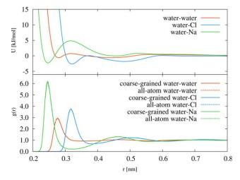
**Figure 9.** Effective pair potentials for water–water, water–Cl, and water–Na are shown on top. Radial distribution functions for an all-atom and coarse-grained simulations are shown at the bottom. Atomistic RDFs are very well reproduced by the coarse-grained simulation.
