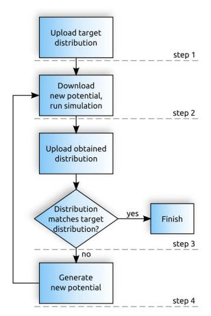
Figure 4. Usage diagram for the Boltzmann inversion tool. Steps 2, 3, and 4 are iterated until the coarse-grained distribution matches the target distribution. Simulation in step 2 is run locally on one's machine. [Color figure can be viewed in the online issue, which is available at wileyonlinelibrary.com.]
