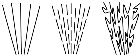
Fig. 1 Schematics of splay deformation. For long chains (left), the density decreases as the chains spread out, shorter chains (middle) possess more ends and can fill the voids more easily. Backfolds (right) also fill the voids, but reduce orientational ordering unless they are pointlike U turns (hairpins), which are favoured in the nematic phase. In this case, they act as chain ends and can fill the voids similar to the middle picture.
