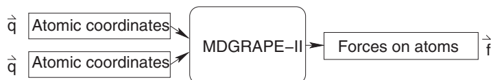
Fig. 10.7 The calculation of forces by the MDGRAPE-II. The atomic position vectors \mathbf{q} are input, and the MDGRAPE-II returns a vector of forces \mathbf{f} exerted on the atoms.
